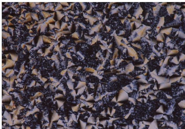
Figure 6. Optical textures observed for BOXD-T14 at (a) 10 °C ( \times 200 ) on the cooling run.
